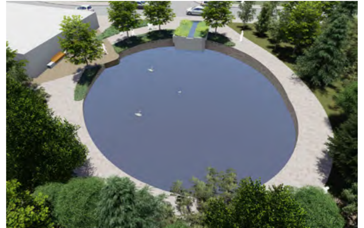
Illustrative view of balancing pond for attenuation
